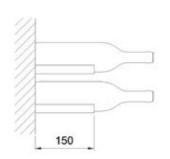
V-PINS: The V-Pins are used to hold the wine bottle in a cork facing direction. Maximum storage capacity gained from this method. Shared central pin. i.e 3 pins to hold 2 bottles.
