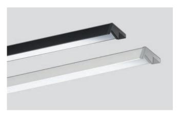
Cuttable to size oxidized aluminium profile for surface mounting with glare cover; available in Aluminium or Black finish; it combines with a cuttable to size opal polycarbonate screen cover, and end caps with cable lock. Installation by means of fixing screws (not included).
