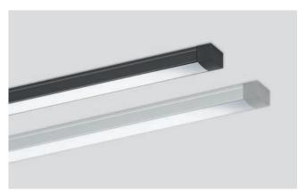
Cuttable to size oxidized aluminium profile for surface mounting, available in Aluminium or Black finish; it combines with a cuttable to size opal polycarbonate screen cover, and end caps. Installation by means of polycarbonate fixing clips or double-sided tape (not included).
