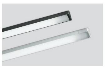
Cuttable to size oxidized aluminium profile for surface mounting, available in aluminium or painted black finish; it combines with a cuttable to size polycarbonate screen cover (opaline) and end caps with cable locking clips; installation by means of double-sided tape (not included).
