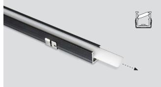
$\ensuremath{\textcircled{\textbf{1}}}$  Remove the wired power connector
