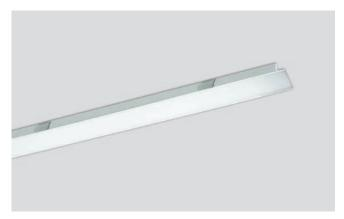
Cuttable to size oxidized aluminium profile for recessed mounting; it combines with a cuttable to size polycarbonate screen cover (opaline); installation by means of fixing clips (plastic adhesive cable clamp included).
